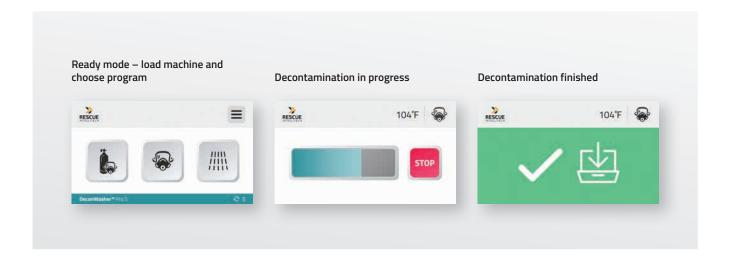
To make the machine as user-friendly as possible, we decided to use a single resistive touch screen display, so you have complete control of your DeconWasher Pro S. With a modern user interface, inspired by the easy-to-use analog control panel of the Solo Rescue, you can run a wash program with a single tap on the screen.
